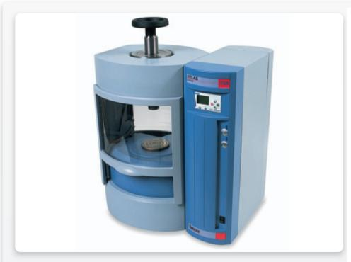
The Atlas™ Power Presses T8, T15 & T25, are power assisted hydraulic presses operating to 8, 15 & 25 Tons respectively.
