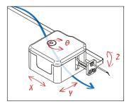
The different operating modes of the piezo actuators provide up to centimeters travel range with **scalable positioning resolution from micrometers to nanometers**. The coarse positioning mode saves time when approaching the region of interest, while the fine positioning mode allows for a precise contact landing of the probes at the destination.
