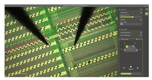
Precisio $^{\text{TM}}$  software microscope window with controls for imaging parameters, tools for recording, annotation, and dimensional measuring.
