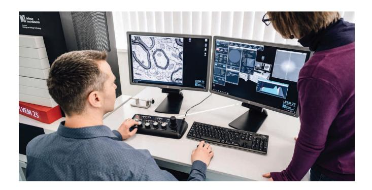
The LVEM 25 produces images with unmatched contrast from your conventionally prepared samples. Three powerful imaging modes are available in a single compact instrument. Switching between imaging modes is done easily via operating software, providing quick image collection of the same region of interest in TEM, STEM and ED modes.
